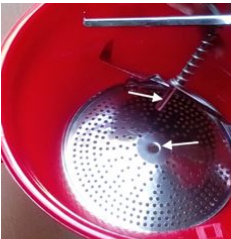
3. Insert the handle pivot into hole in disc
