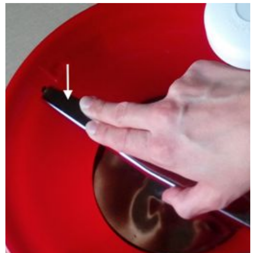
5. To change disc or disassemble the food mill press bar down and rotate it to remove hooks from seats
